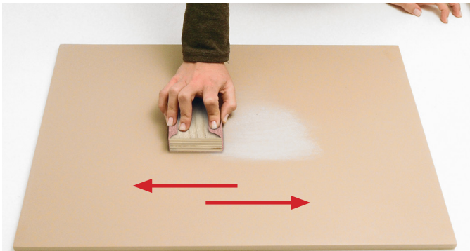
3. Widen the chipped area with a wooden block (D) and P180 sandpaper (A) in order to remove all the scratches or stains.
