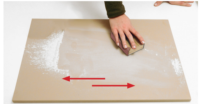
4. Sand the surface with the wooden block (D) and the P240 sandpaper (B) following the direction shown above to restore the surface partially.
