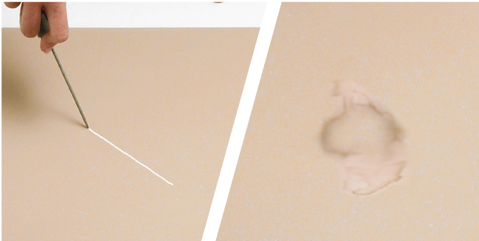
1. Scratched or stained surface.
