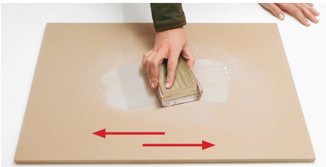
5. To fulfill the complete restoring on the surface, use the wooden block (D) with the sandpaper P320 (C).
