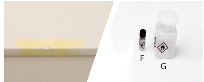
4. Circumscribe the area to be repaired with masking tape, then pour the whole catalyst (F) in the Gelcoat flask (G) and stir until a homogeneous blend is obtained.
