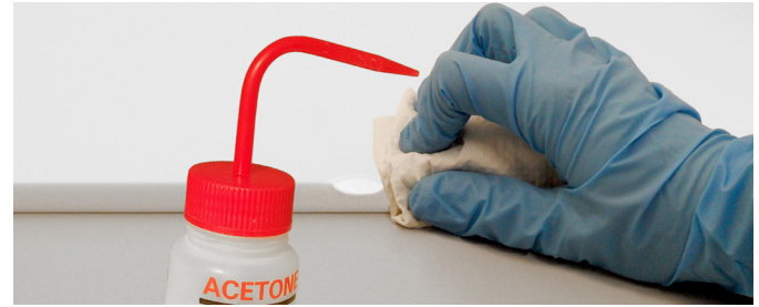
4. Remove dust and clean the surface with acetone or alcohol.
