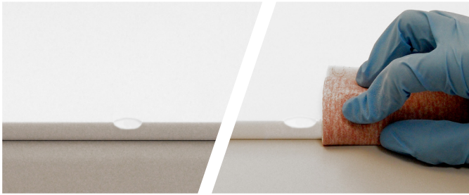
3. Widen the chipped area with the wooden block (H) and P180 sandpaper (A) in order to smooth the surface and remove all small cuts. Polish the surface next to the damaged area with 320-grit sandpaper (C).
