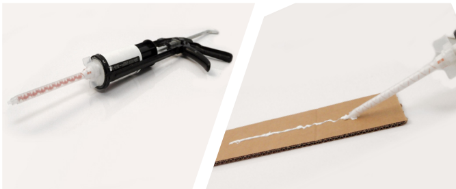
5. Remove the cartridge cap (F), cut its top, and introduce the stirring stick (G). Load a silicone gun with the cartridge and take care to discard the first 10 cm of product.
